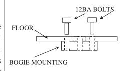
has been fixed in place) either side of the bogie pivot bolt, tap 12BA. Now secure the bogie pivot in place by bolting down through the coach floor with short 12 BA bolts.
